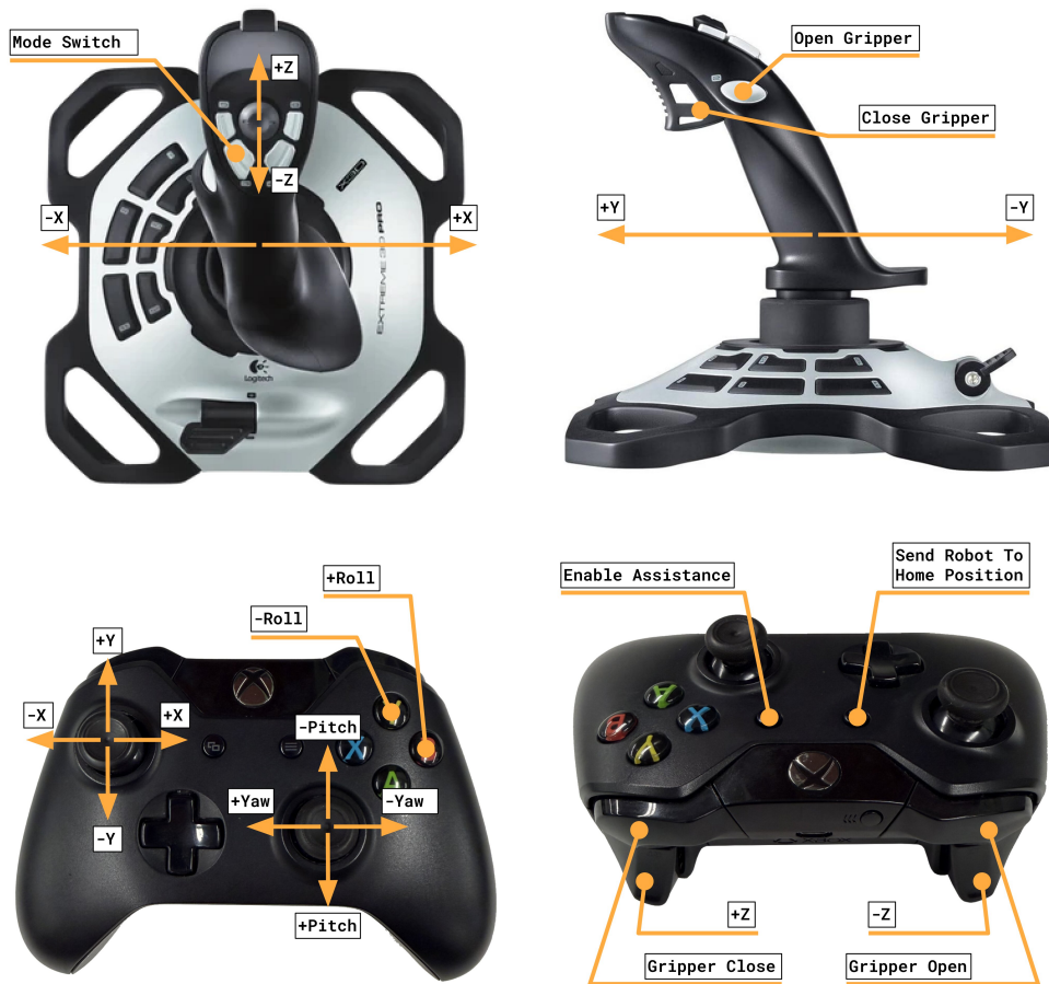
Figure 3.4: Control devices used in the study. Top row : Logitech Extreme 3D Pro Joystick interface used by study participants. Bottom row : Xbox 360 controller used by the author during demonstrations.
